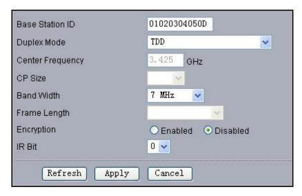
Figure 10 ZMAX-8210 Wireless Parameters
